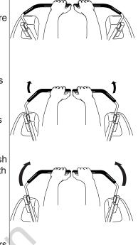
Figure 3. Move Control Levers Gradually
